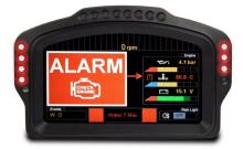
The ICD features super bright, fully configurable tricolour LED arrays for multi-purpose use as alarms, shift lights, driver aids etc. together with an in-built LDR for auto LED and screen brightness control.
